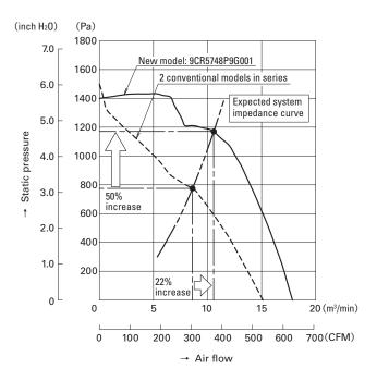
Fig. 5: Air flow vs static pressure characteristics (comparison between the conventional model and the new model)
