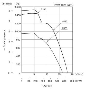
Fig. 3: Air flow vs. static pressure
