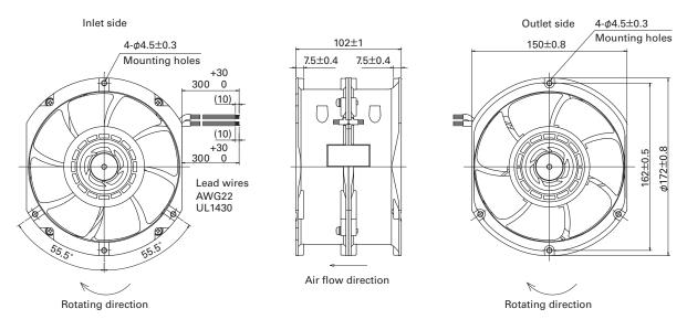
Fig. 2: Dimensions of the new model (unit: mm)
