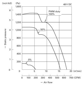
Fig. 4: Air flow vs static pressure characteristics at individual PWM duty cycle
